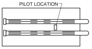
TOP VIEW OF BURNER ASSEMBLY
